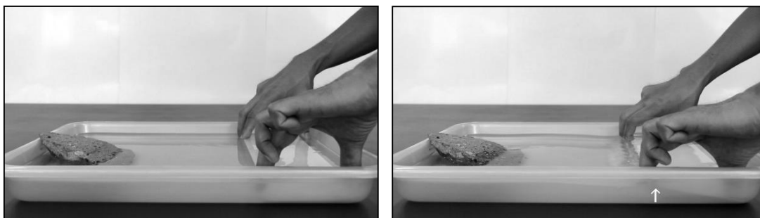
Figure 16. (Left) The plastic panel placed flat at the bottom of the container. (Right) Wait for the water to stop moving, then suddenly jerk the edge of the plastic panel upward (see white arrow).
