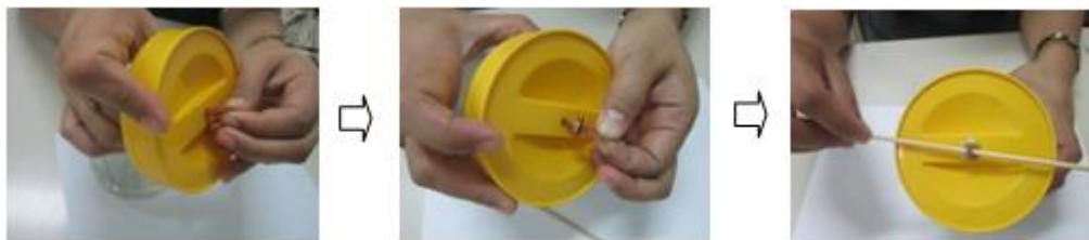
Figure 9. Steps in inserting the bead and the long barbecue stick
